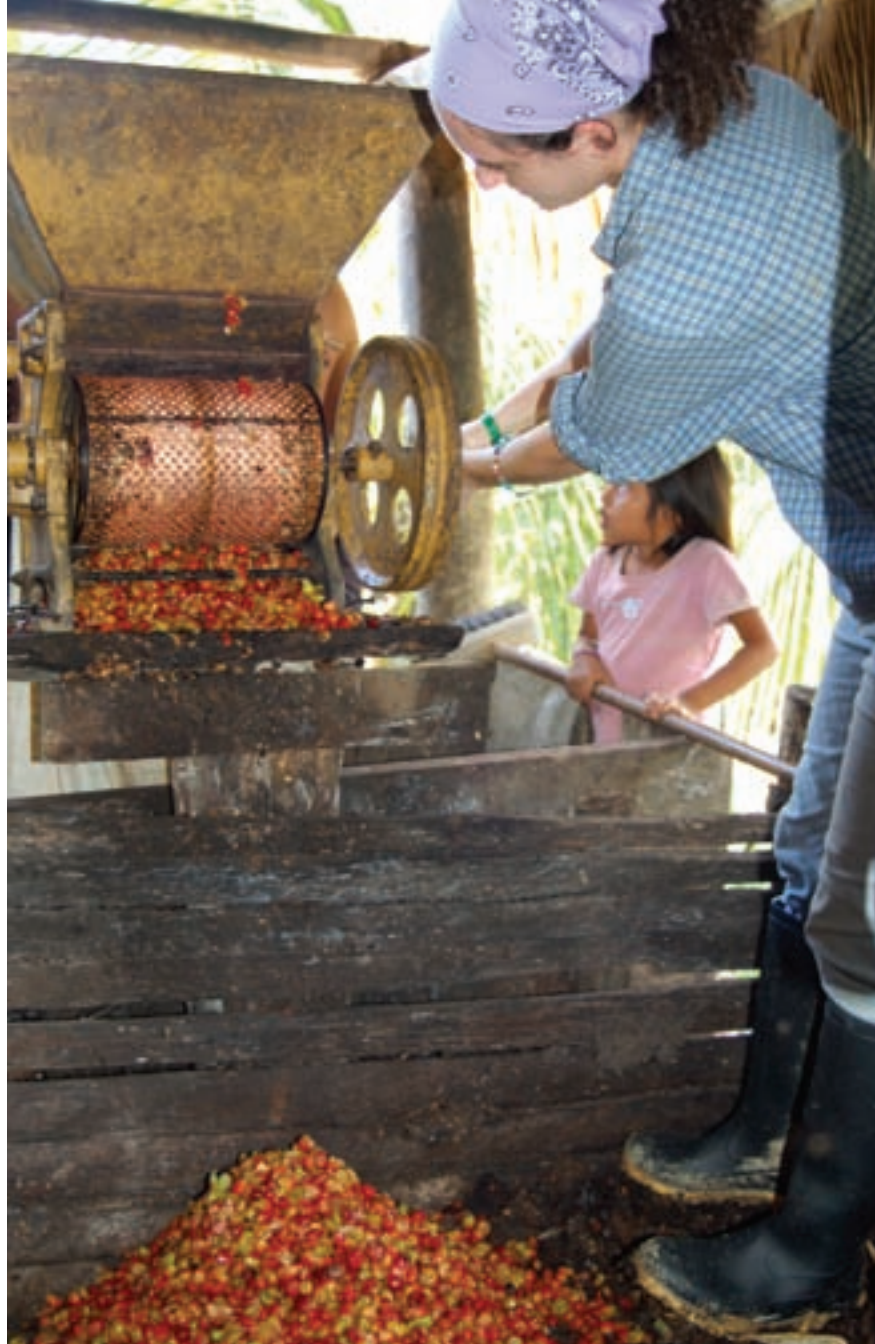
Zoe Kantor using a coffee depulper to separate the cherry, the red rind surrounding the coffee bean, from the coffee bean itself. The machine has made a huge difference to the town of Alto Chambuyaco and was purchased through increased profits from joining the fair trade coffee cooperative "Oro Verde," Living Routes' partner organization for the fair trade and biocultural regeneration in the high Amazon.
